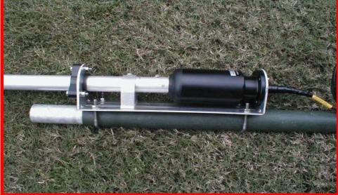
• The bottom picture shows the base of the antenna mounted to an aluminum mast section. Notice the exceptionally small matching network (black cylindrical section) of the antenna. No extended radials, this is it!
