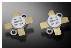
200-Watt Version Utilizes Push-Pull SD2931 Devices
