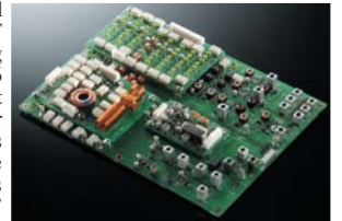
●RX Unit (Showing the VRF and BPF Units)
