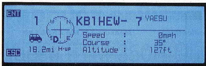
Figure 1 — Two examples of the FTM-350R display during APRS operation. (Left) Received positions include an icon, distance, relative location (D), speed and coordinates. (Right) Received weather beacon information can include temperature, precipitation and wind speed.
