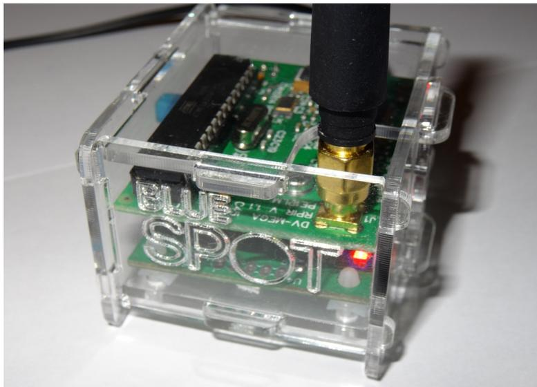
The assembly consists of a DVMega board, to manage the connection with the D-Star / DMR / C4FM and the digital walkie talkie, then the Bluestack Micro+ board to manage the connection via Bluetooth with the Android smartphone (or the tablet) connected to a wi-fi or 3G/4G internet connection, to send radio traffic online.
