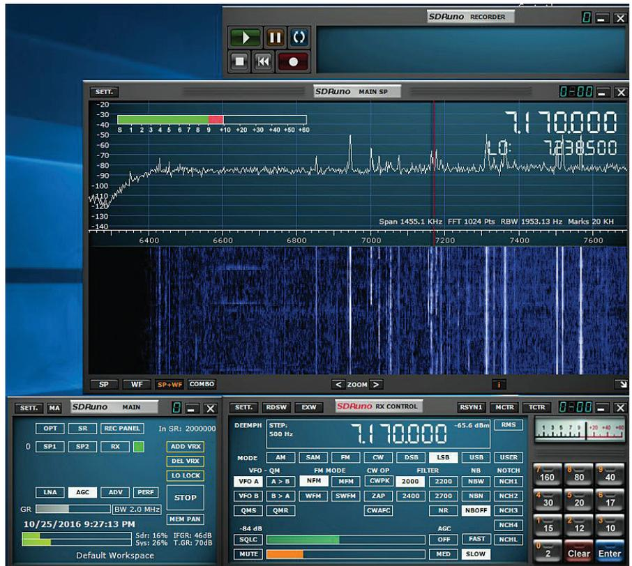
Figure 7 — RSP1 receiving on 40-meter SSB using SDRplay software. Only one receiver is shown here, but the application can open several simultaneously.
