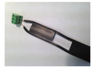
Also, in practice a short length of coax can be terminated directly to the outer terminal connections of the supplied CTB9208/3 plug, without significant loss of signal. Losses due to mismatch are small if the length of the coax is kept well below 1/4 wavelength at the frequency of interest.
