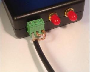
The short length of coax can be terminated with a suitable flying socket (e.g. BNC for use with active loop antennas or SO239 for connection to other existing LF antenna choices.
