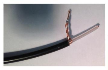
Connect the coax inner to the P terminal and the outer to the N and GND terminals as in this example which is using a short length of RG58
