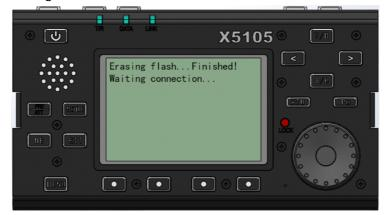
Note: Don't unplug the power cable during the erasing process.
