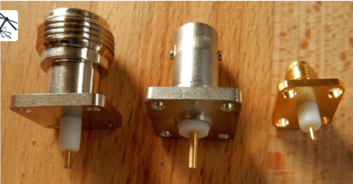
Figure 13 - Examples of suitable panel mount flanges
