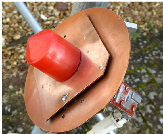
Another approach is to produce a lens yourself on a lathe. The pictures below show an experimental lens, made from 20mm diameter Nylon-6 (PolyAmide 6, or PA6). The final dimensions of the lens is still work in progress.
