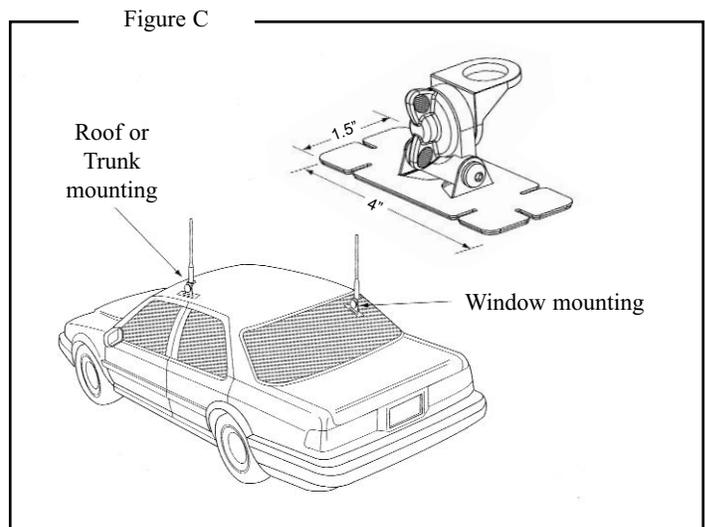
4. Route coaxial cable from antenna mount to radio.
