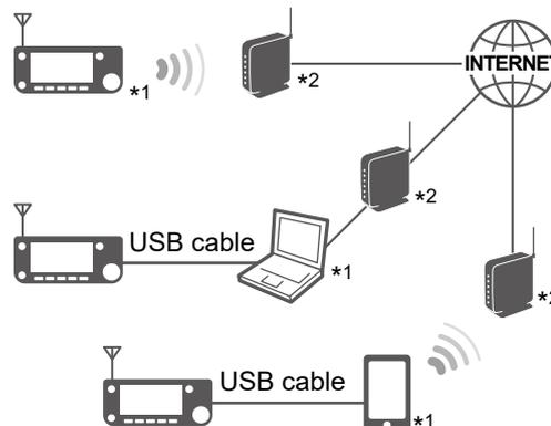
\*1 A static IP address to the transceiver, Windows, or Android device is recommended.
