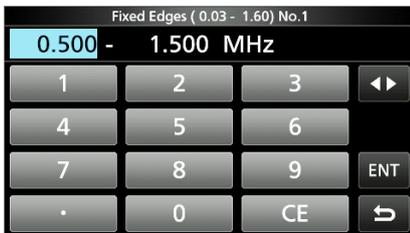
① Touch **◀▶** to select the upper and lower edge frequency, and then rotate **⊕MULTI** or touch the keypad to edit the frequency.
