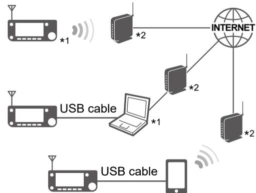
\*1 A static IP address to the transceiver, Windows, or Android device is recommended.
