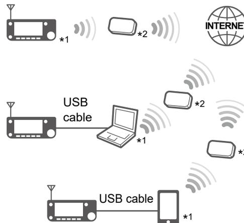
\*<sup>1</sup> A static IP address to the transceiver, Windows, or Android device is recommended.
