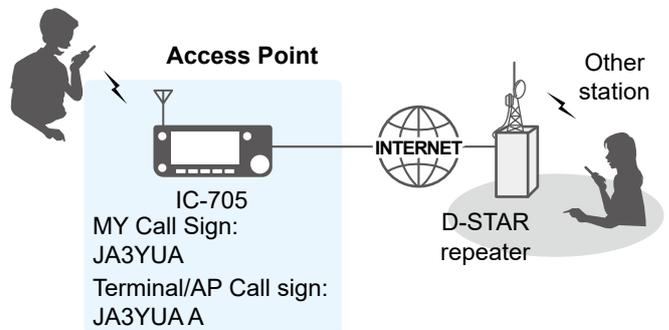
**When using the External Gateway function**
