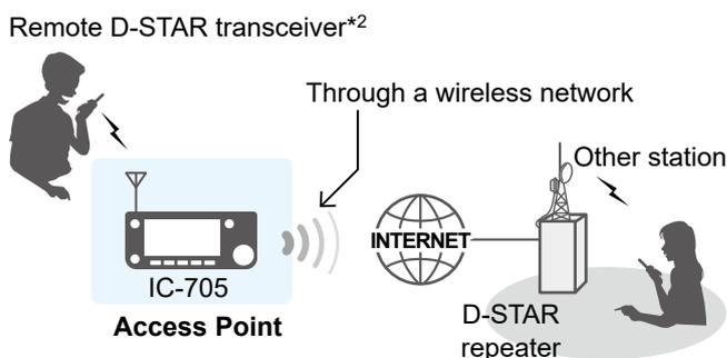
\*<sup>1</sup> Within the transmit and receive range of the Access Point transceiver. The range will vary, depending on the operating environment.
