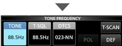
5. Rotate **(MAIN DIAL)** to set the desired subaudible tone frequency.
