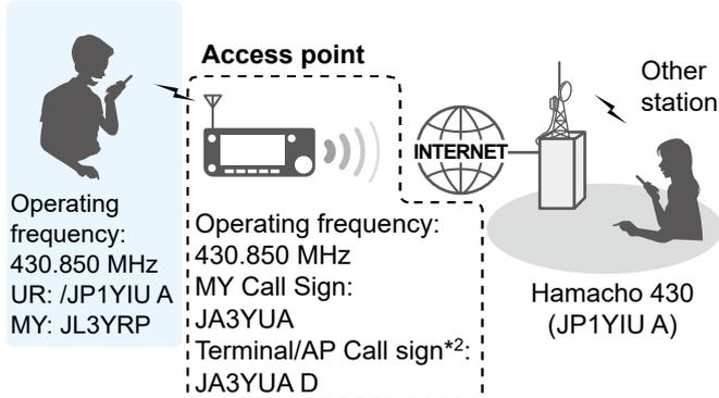
\*1 Any model as long as the transceiver is D-STAR capable. Only one D-STAR transceiver can use the Access Point at the same time.
