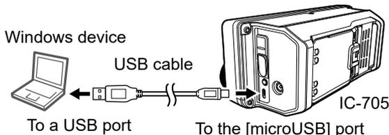
**NOTE:** Turn OFF the transceiver before connecting or disconnecting the cable.
