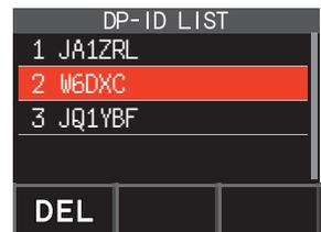
2. Rotate the DIAL knob to select the call sign of the other transceiver, then touch **[DEL]**.
