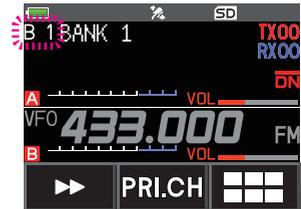
The memory bank channels are displayed between the memory channel 1 (1CH), and PMS memory channel U50.
