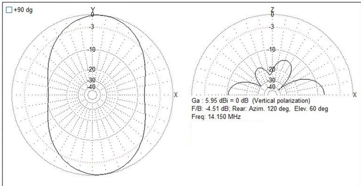
Figure 15. Inverted "V" Far Field Plot 14 MHz.
