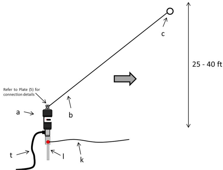
**Figure 4. Sloping Wire Configuration.**
