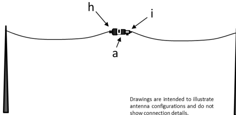
**Figure (7). Horizontal Dipole.**
