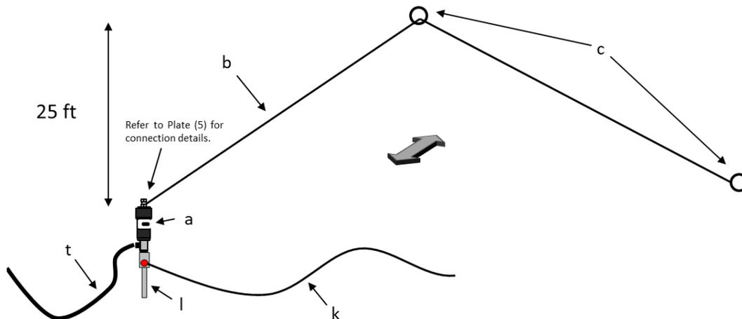
Figure 6. Inverted "V" Configuration.
