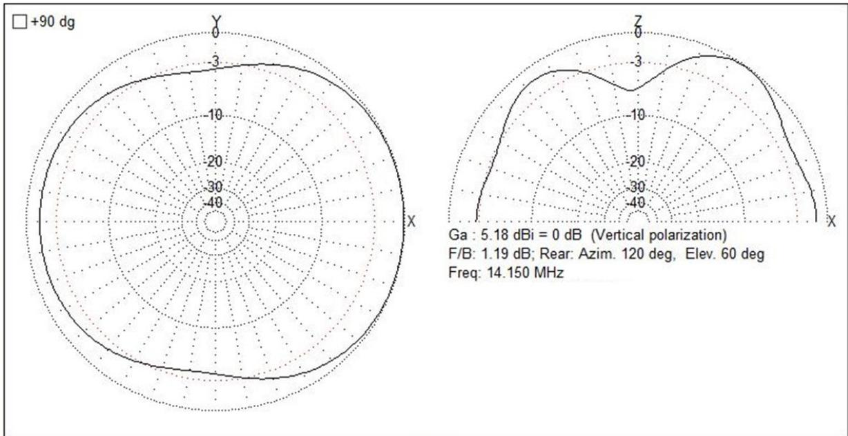
Figure 13. Sloping Wire Far Field Plot 14 MHz.
