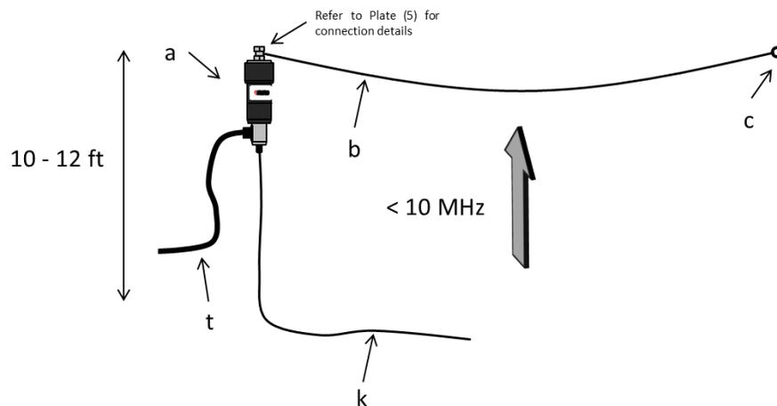
**Figure 3. Horizontal NVIS Configuration.**
