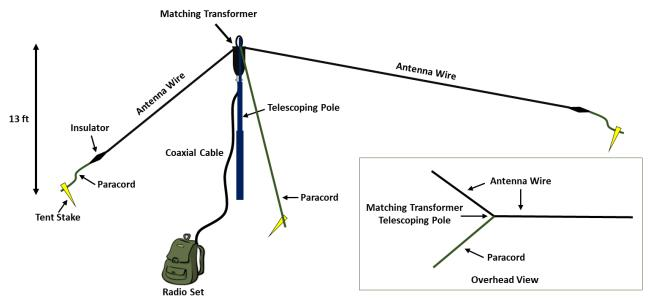
Figure 3. Self-Supporting 40 Meter OCFD Field Installation.
