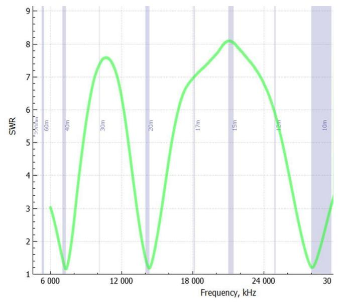
Figure 4. 40 Meter OCFD SWR by Frequency.
