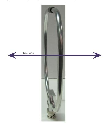
The Loop Antenna has the advantage of being less affected by reflection signals due to its Faraday shield.
